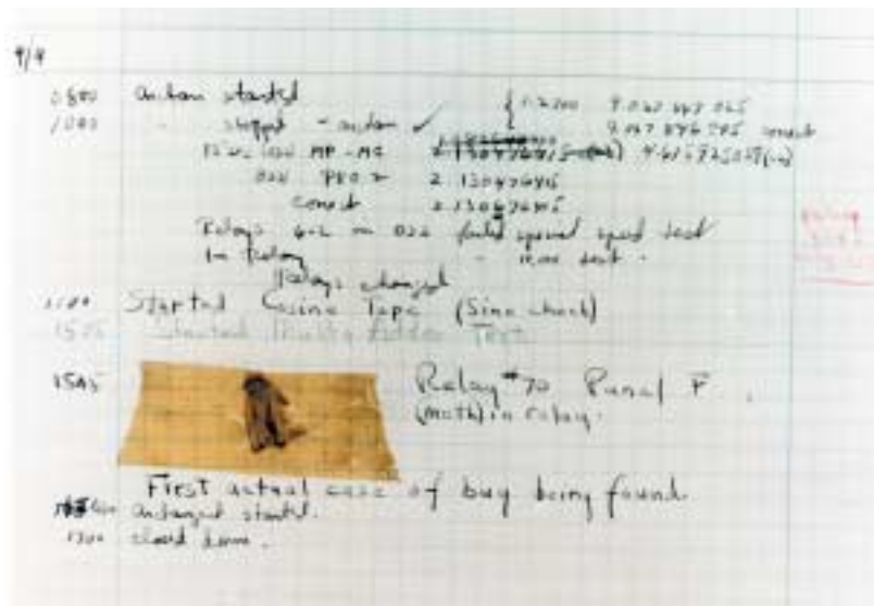
The first computer bug. In 1945, a moth was removed from Relay #70, Panel F, of the Harvard University Mark II Aiken Relay Calculator.
